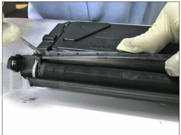
4. Using a flathead screwdriver, pry loose the doctor blade cover from either side of the toner cartridge as shown.
