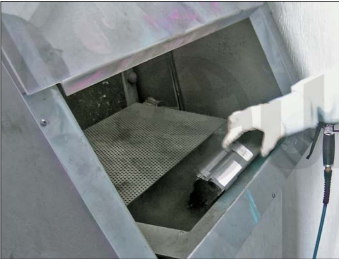
19. Gently tap out the cartridge to empty out the residual toner.
