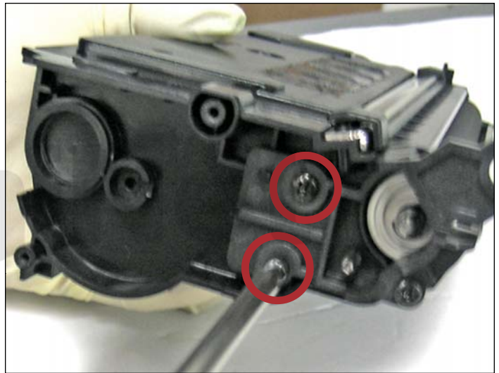
6. Remove the two developer roller support screws shown from the gearless side of the cartridge.
