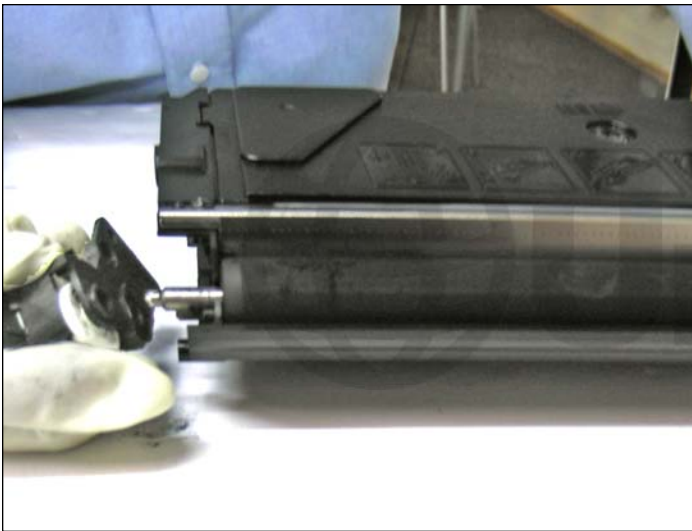
7. Gearless side developer roller support removed.
