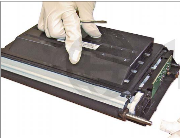
5. Remove the gears from each side. They should slip off fairly easily.
