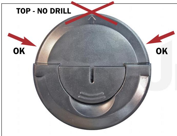
5. In order to clean and fill the cartridge with new toner, we must first create a small hole by drilling through either side. The hole must then be sealed with a fill plug adhesive or sealing tape.
