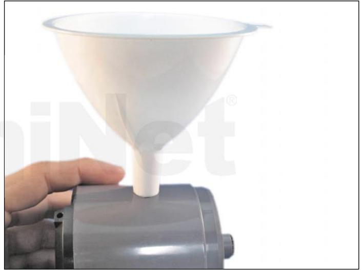
9. Insert a funnel through the hole. Be sure to shake the toner bottle well before opening. Pour the appropriate amount of toner via the funnel.
