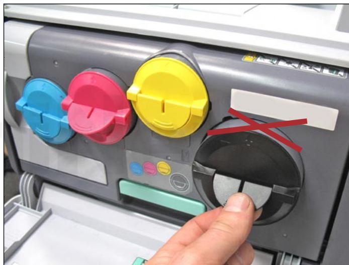
6. Do not drill or place any seal or adhesive on/near the top area of the cartridge. The space between the top surface of the cartridge and the housing wall just above it is very tight. Friction or rubbing while inserting the cartridge can cause the seal to loosen or break off and lead to toner leakage.
