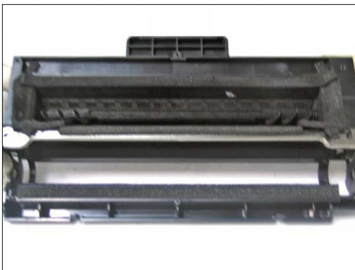
11. PCR and OPC drum removed.
