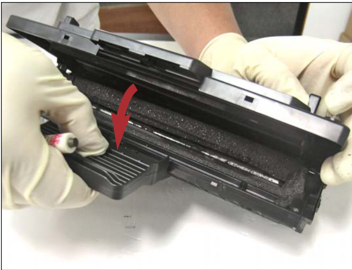
3. Open the cartridge cover as shown.
