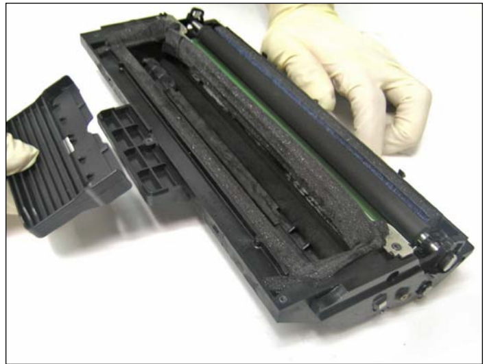
4. Remove the extension handle.
