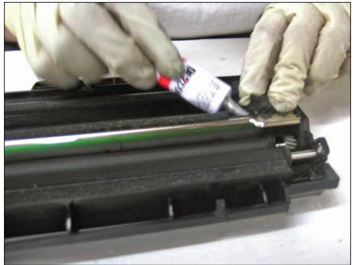
22. After you have reinstalled the components, use a rubber adhesive to bond the foam seal back in its original place. Bonding the foam will prevent leaks.
