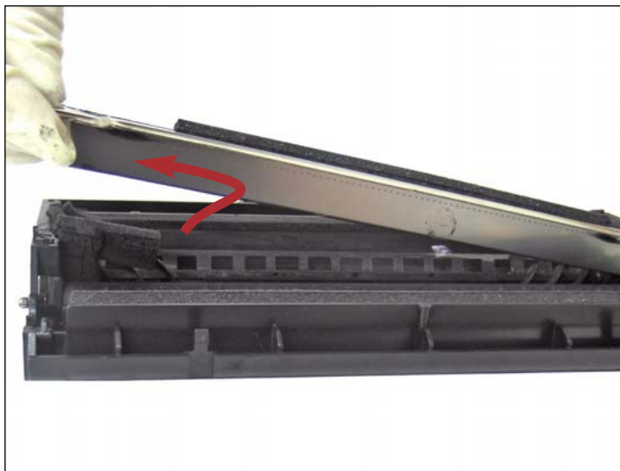
14. Lift the blade up, then slide out as shown.
