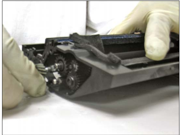
16. Remove all gears as shown.
