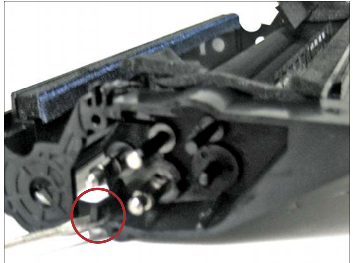
18. Remove the roller support plate by releasing the first clip located under the developer roller axle.
