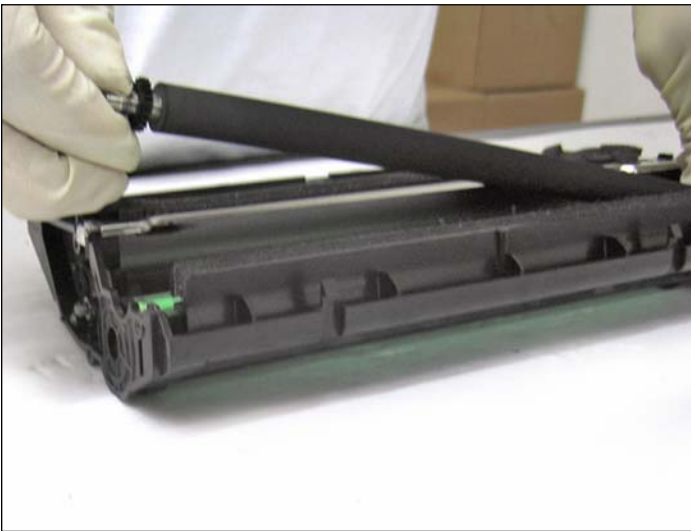
7. Remove the PCR as shown.
