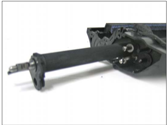
20. Remove the support plate and pull out the developer roller.
