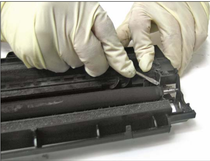
19. Release the second clip located at the opposite end just above the developer roller.
