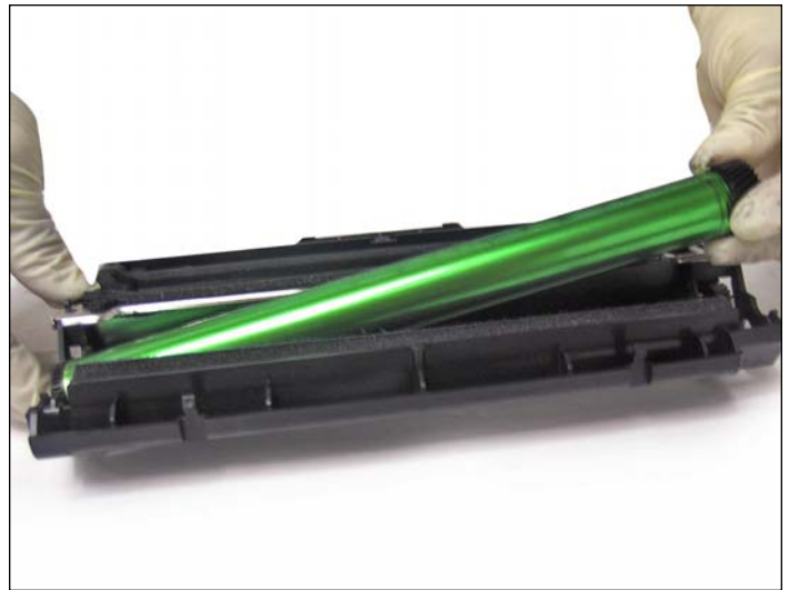
10. Remove the drum as shown.
