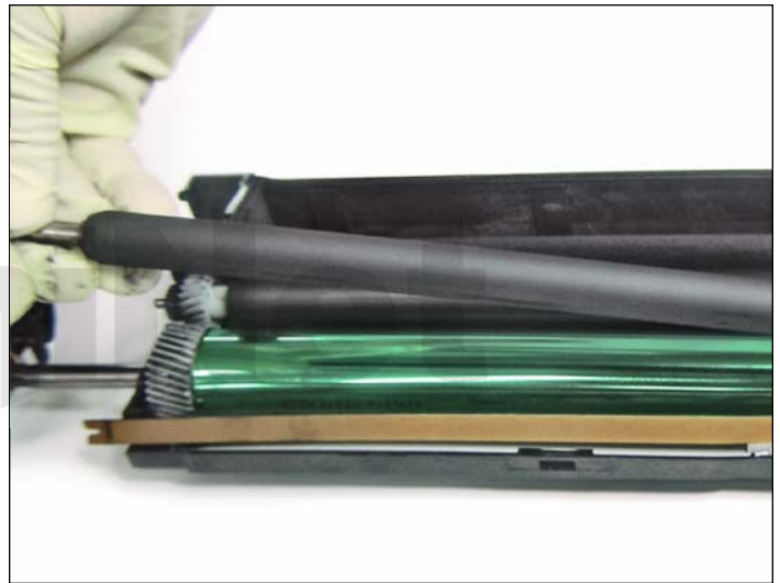
11. The PCR can now be removed.
