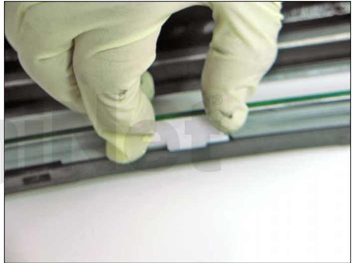
19. Remove the drum erase lamp holder by pulling it out.
