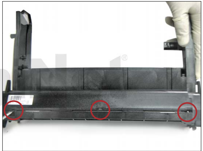
4. Using a small flathead screwdriver, press the five tabs on the back and front of the cartridge to release the drum unit cover.
