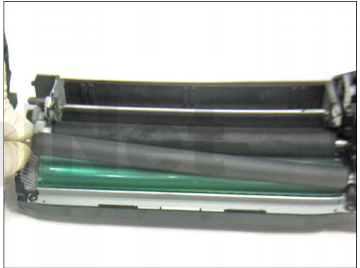
9. Partially slide the end cap with the connected drum axle by about two inches.
