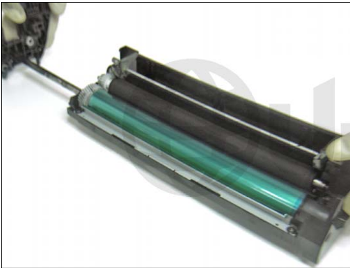
10. Slide the end cap and drum axle out completely.
