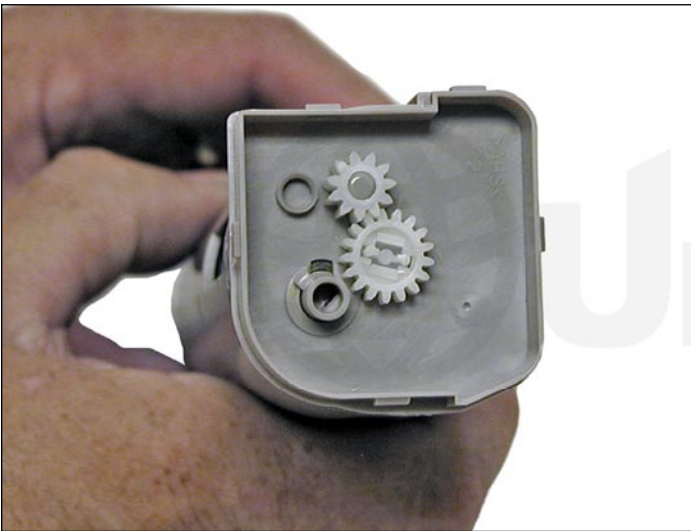
10. Replace the center section into the supply section and snap the drive gear in place. Replace the smaller gear.
