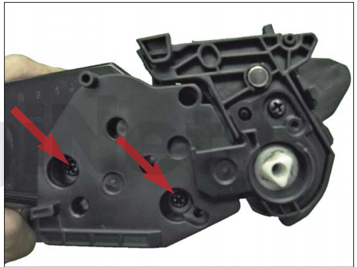
17. Install the P2015 right end cap.
