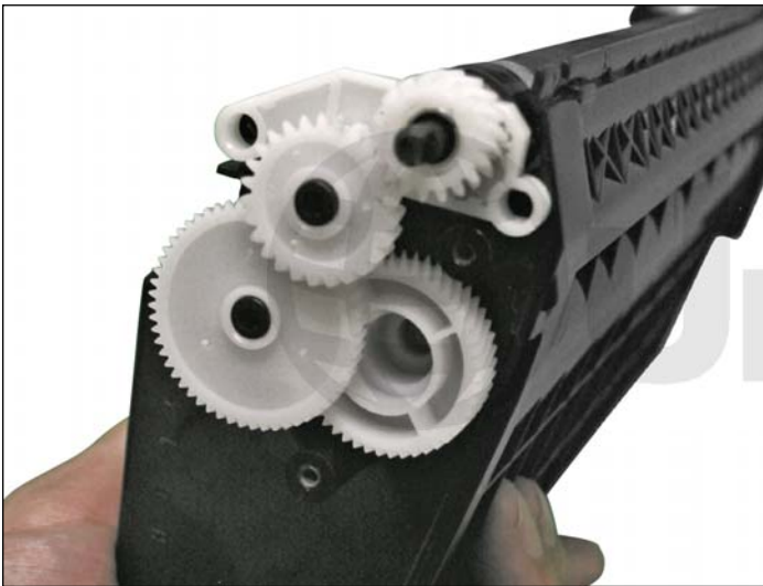
16. Install the magnetic roller, the right stabilizer, and all drive gears on the right side of the hopper as shown.
