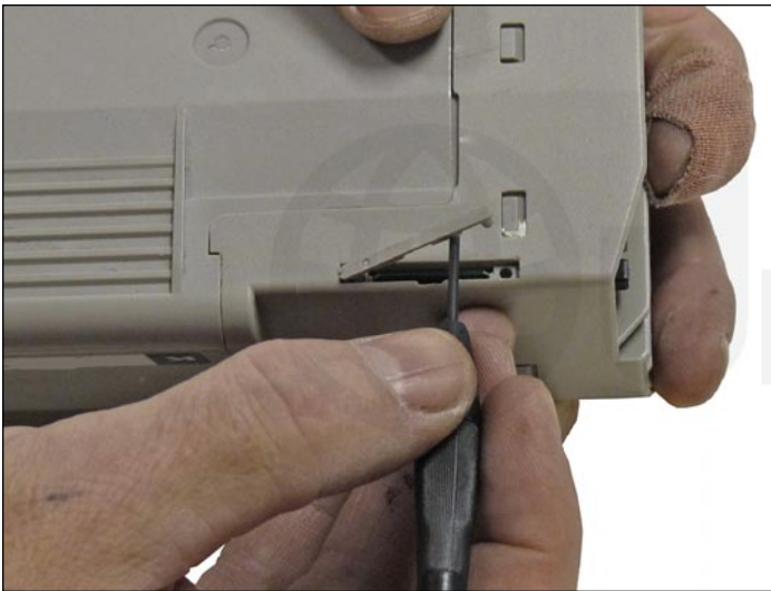
7. Carefully pry-up the chip cover from the hopper. It is best to remove the end closest to the edge of the cartridge first to help prevent any damage to the cover tabs.
