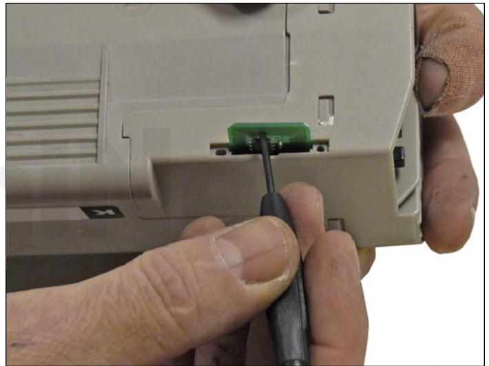
8. Remove the old chip and install the new. Be sure to keep the component side up when replacing the chip.
