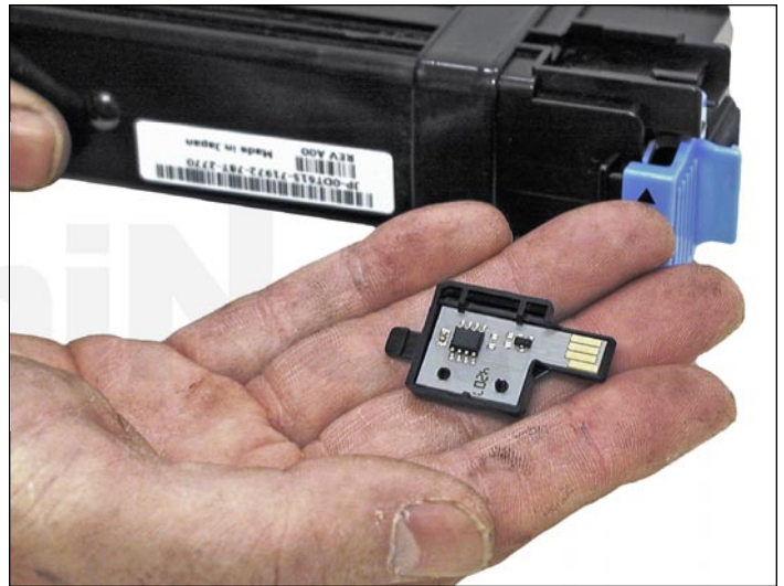
9. Slide the holder out of the cartridge and replace the chip.
