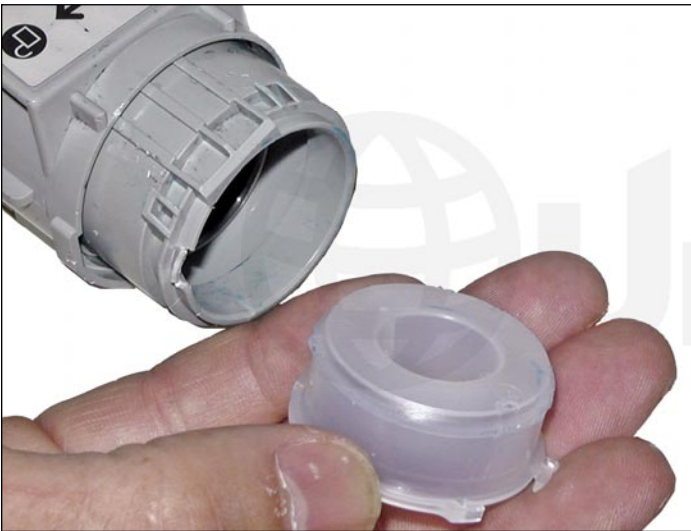
3. Very carefully pry out the fill plug It is very soft and easily damaged!
