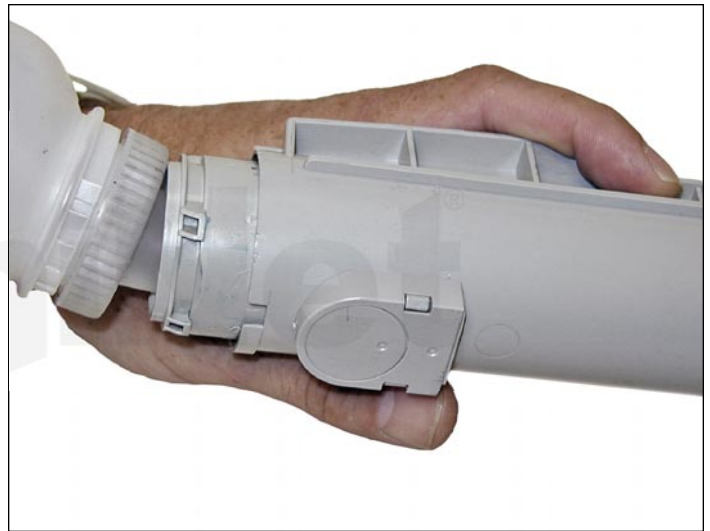
4. Remove all the old toner and fill with new Dell 5100CN toner.
