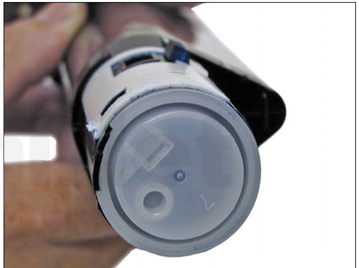
4. Remove the fill plug on the end of the cartridge.
