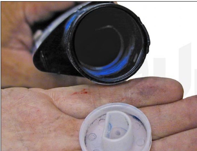
5. Take a screwdriver and insert it through the toner port. Press against the inner fill plug. Remove the plug. Clean out all the remaining toner.
